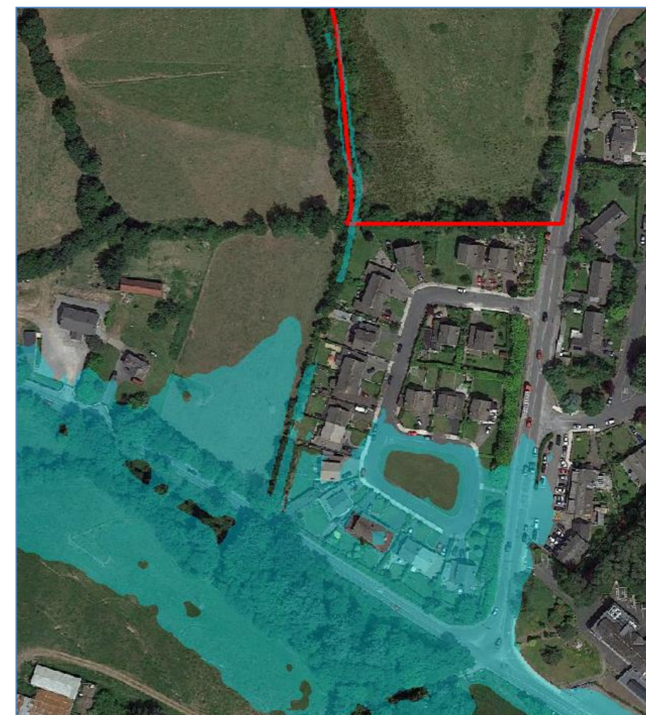
Figure 3.1-Extent of inundation arising from 1%AEPCC peak flow in river and a nominal flow in the western stream (0.2m 3 /s)
